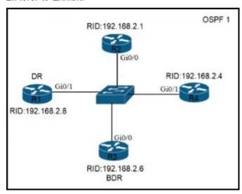
Refer to the exhibit. All routers in the network are configured R2 must be the DR. After the engineer connected the devices, R1 was elected as the DR.
