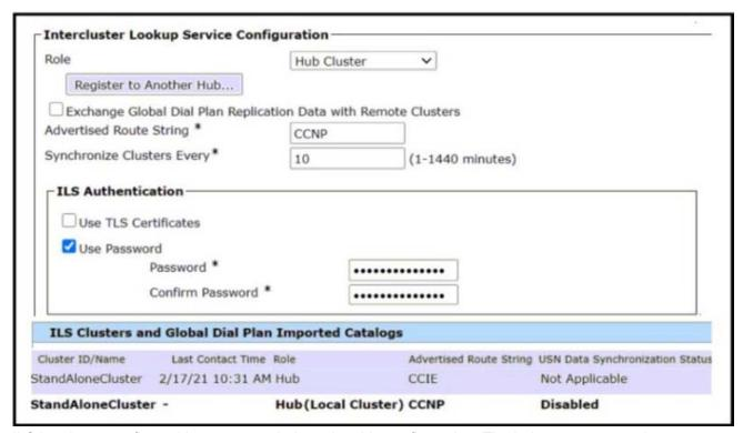
ILS has been configured between two hubs using this configuration. The hubs appear to register successfully, but ILS is not functioning as expected.
