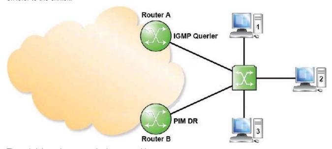
The switch is not igmp-snooping/proxy capable.
