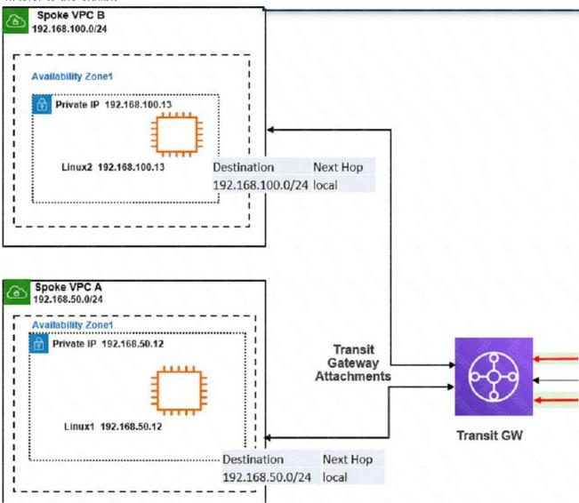
The exhibit shows a customer deployment of two Linux instances and their main routing table in Amazon Web Services (AWS). The customer also created a Transit Gateway (TGW) and two attachments Which two steps are required to route traffic from Linux instances to the TGWQ (Choose two.)
