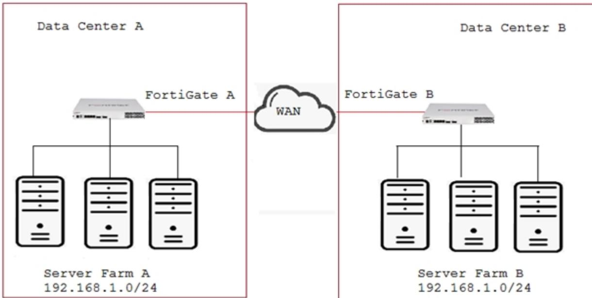
Your company has two data centers (DC) connected using a Layer 3 network. Servers in farm A need to connect to servers in farm B as though they all were in the same Layer 2 segment.
